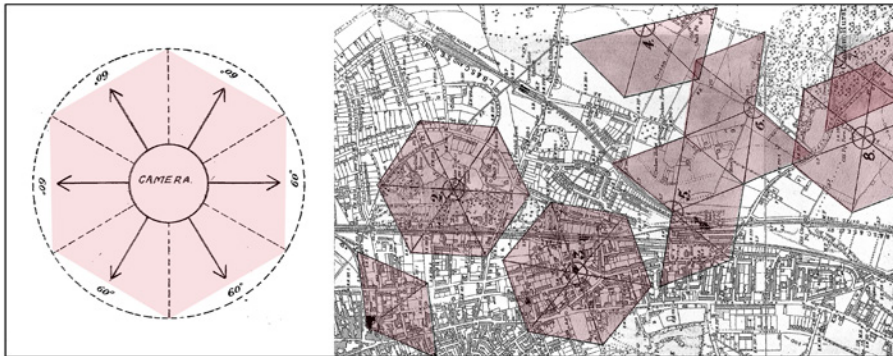
Fig. 6.1 (left): A diagram representing the controlled rotation of the camera at each selected point within a grid.
